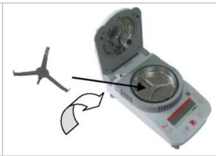
(2) Install Pan Support, turn until it engages into position
